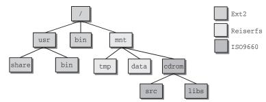
Figure 8-4: Filesystem hierarchy with various filesystem types.
