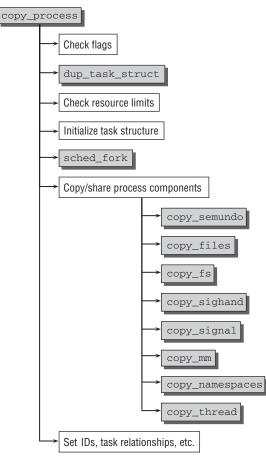
Figure 2-8: Code flow diagram for copy\_process.
