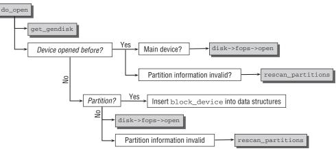
Figure 6-14: Code flow diagram for do\_open.
