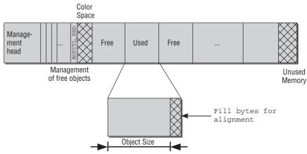
Figure 3-46: Fine structure of a slab.
