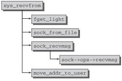
Figure 12-33: Code flow diagram for sys\_recvfrom.
