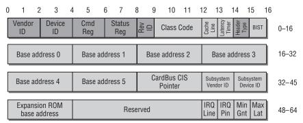
Figure 6-23: Layout of the PCI configuration space.
