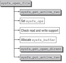
Figure 10-13: Code flow diagram for sysfs\_open\_file.
