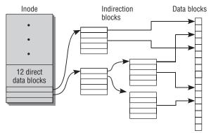
Figure 9-4: Simple and double indirection.
