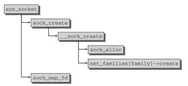
Figure 12-32: Code flow diagram for sys\_socket.
