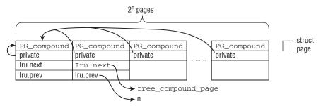
Figure 3-33: Higher-order allocations generate compound pages in which the individual pages are linked.
