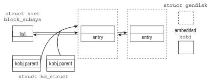
Figure 6-11: Integration of generic hard disks with the generic kernel object framework.
