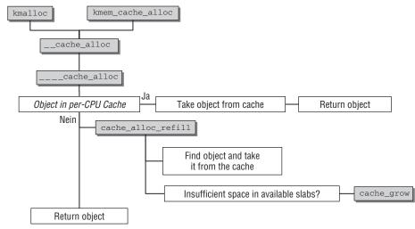
Figure 3-50: Code flow diagram for kmem\_cache\_alloc.
