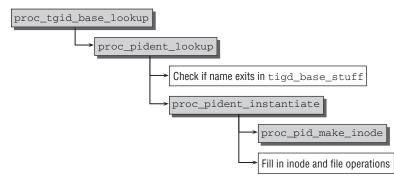
Figure 10-5: Code flow diagram for proc\_tgid\_base\_lookup.
