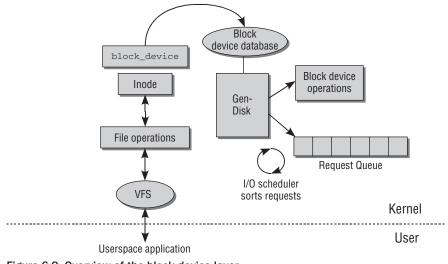
Figure 6-9: Overview of the block device layer.
