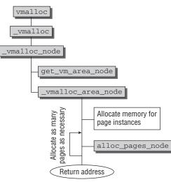
Figure 3-39: Code flow diagram for vmalloc.
