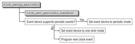
Figure 15-10: Code flow diagram for tick\_setup\_periodic.
