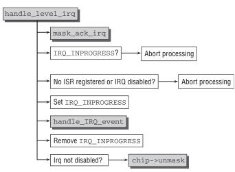
Figure 14-6: Code flow diagram for handle\_level\_irq.
