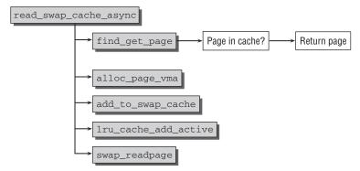
Figure 18-20: Code flow diagram for read\_swap\_cache\_async.
