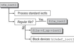
Figure 6-19: Code flow diagram for sys\_ioctl.
