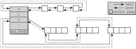
Figure 3-22: Linking blocks in the buddy system.
