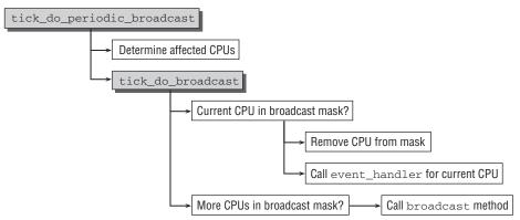
Figure 15-22: Code flow diagram for tick\_do\_periodic\_broadcast.
