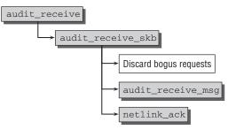
Figure 19-3: Code flow diagram for audit\_receive.
