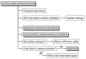
Figure 9-17: Code flow diagram for alloc\_new\_reservation.
