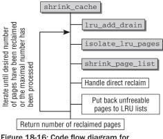
Figure 18-16: Code flow diagram for shrink\_cache.
