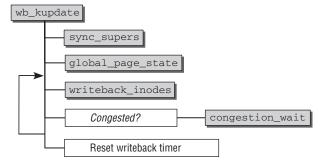
Figure 17-4: Code flow diagram of wb\_kupdate.
