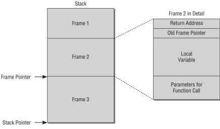
Figure C-1: Activation records on the stack.
