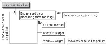
Figure 12-13: Code flow diagram for net\_rx\_action.
