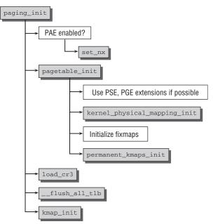
Figure 3-16: Code flow diagram for paging\_init.
