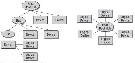
Figure 6-24: Topology of a USB system.
