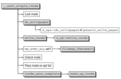
Figure 17-8: Code flow diagram for \_\_sync\_single\_inode.
