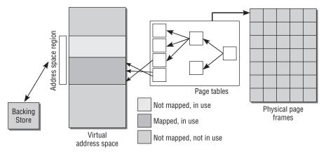
Figure 4-5: Interaction of data structures during demand paging.
