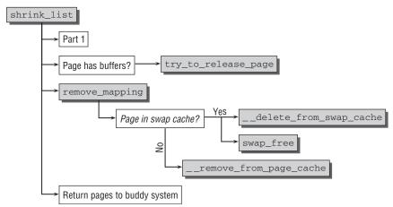
Figure 18-18: Code flow diagram for shrink\_list (Part 3).
