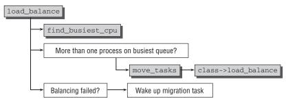
Figure 2-26: Code flow diagram for load\_balance.
