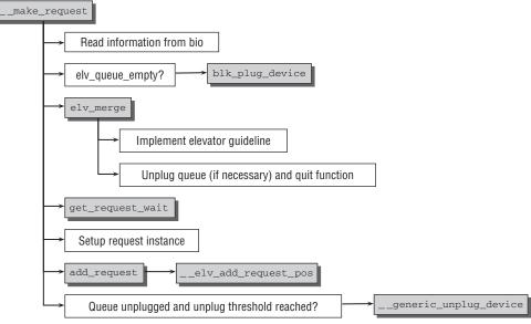
Figure 6-18: Code flow diagram for \_\_make\_request.
