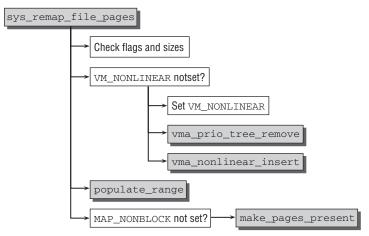
Figure 4-15: Code flow diagram for sys\_remap\_file\_pages.
