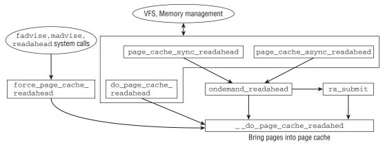
Figure 16-5: Functions used to implement readahead. Note that the figure shows the connections between the functions, but is not a proper code flow diagram.
