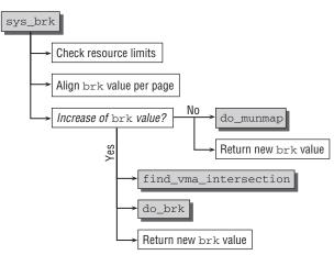
Figure 4-16: Code flow diagram for sys\_brk.
