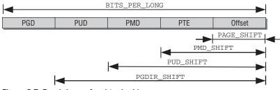
Figure 3-7: Breakdown of a virtual address.
