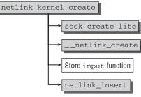
Figure 12-36: Code flow diagram for netlink\_kernel\_create (multicast handling is omitted).
