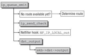
Figure 12-18: Code flow diagram for ip\_queue\_xmit.
