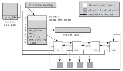
Figure 5-2: Interplay between the semaphore data structures.
