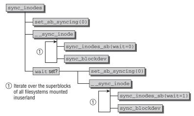
Figure 17-11: Code flow diagram for sync\_inodes.
