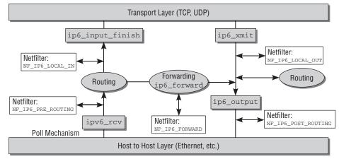
protocols. Changes are apparent, however, when data are passed to the IP layer. Figure 12-22 shows a (coarse-grained) code flow diagram for IPv6 implementation.
