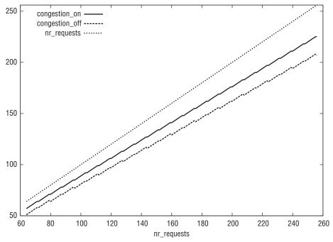
Figure 17-9: Thresholds for the number of requests that turn congestion on and off, respectively. The thresholds are obviously always smaller than the number of requests that can maximally be queued.
