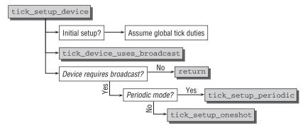
Figure 15-8: Code flow diagram for tick\_setup\_device.
