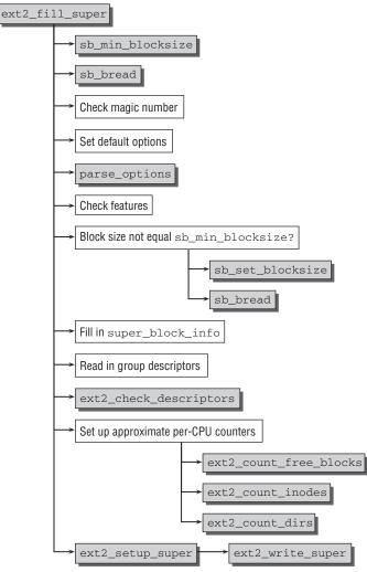
Figure 9-8: Code flow diagram for ext2\_fill\_super.
