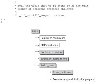
Figure D-3: Code flow diagram for init.
