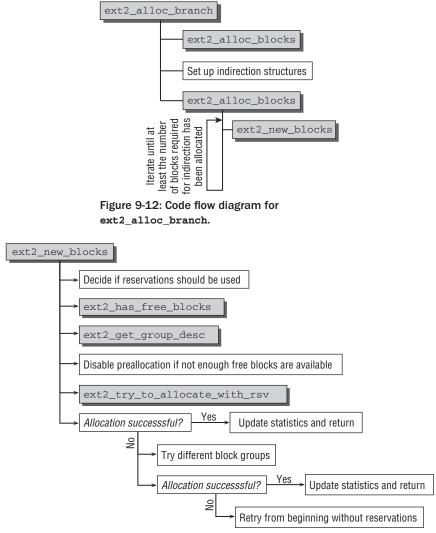
Figure 9-13: Code flow diagram for ext2\_new\_blocks.
