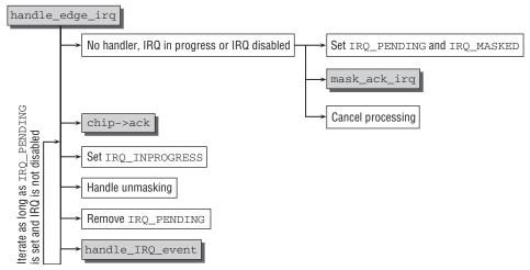
Figure 14-5: Code flow diagram for handle\_edge\_irq.
