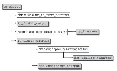
Figure 12-19: Code flow diagram for ip\_output.
