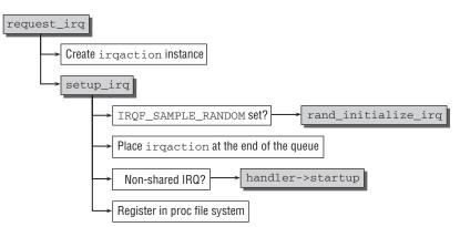
Figure 14-7: Code flow diagram for request\_irq.
