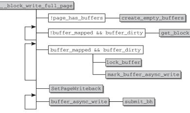
Figure 16-8: Code flow diagram for the buffer-related operations of \_\_block\_write\_full\_page.
