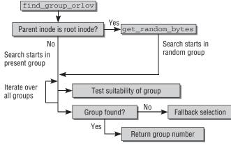
Figure 9-20: Code flow diagram for find\_group\_orlov.
