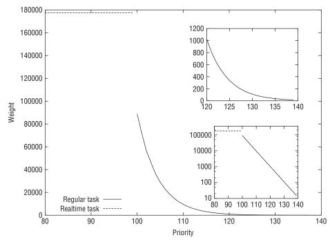
Figure 2-15: Relation between static priority and load for regular and real-time processes.
