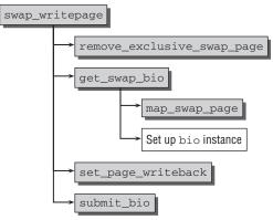
Figure 18-10: Code flow diagram for swap\_writepage.
