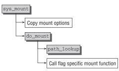
Figure 8-5: Code flow diagram for sys\_mount.
