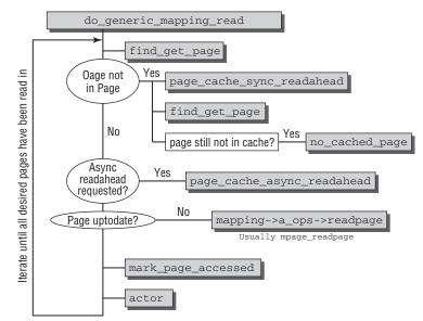
Figure 8-14: Code flow diagram for do\_generic\_mapping\_read.
