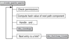
Figure 8-9: Code flow diagram for <u>\_\_link\_path\_walk</u>.
