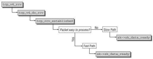
Figure 12-30: Receiving packets in TCP connections.
