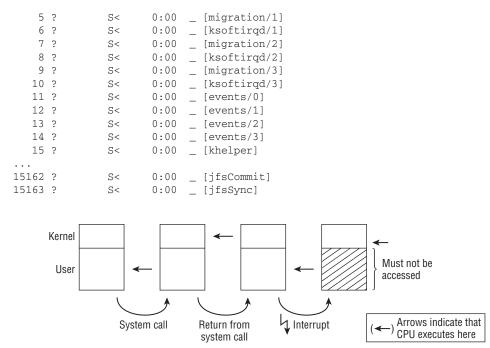
Figure 1-5: Execution in kernel and user mode. Most of the time, the CPU executes code in userspace. When the application performs a system call, a switch to kernel mode is employed, and the kernel fulfills the request. During this, it may access the user portion of the virtual address space. After the system call completes, the CPU switches back to user mode. A hardware interrupt also triggers a switch to kernel mode, but this time, the userspace portion must not be accessed by the kernel.
