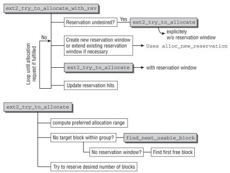
Figure 9-14: Code flow diagram for ext2\_try\_to\_allocate\_with\_rsv.
