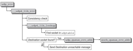
Figure 12-23: Code flow diagram for udp\_rcv.
