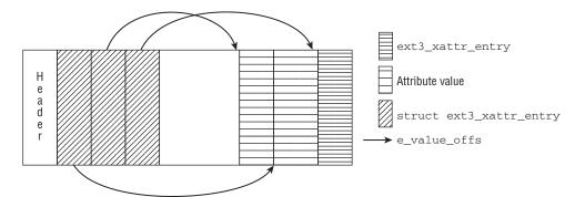
Figure 11-4 presents an overview of the on-disk layout of Ext3 extended attributes.
