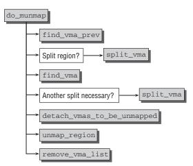
Figure 4-13: Code flow diagram for do\_munmap.
