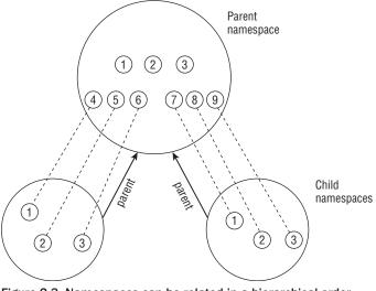
Figure 2-3: Namespaces can be related in a hierarchical order. Each namespace has a parent from which it originates, and a parent can have multiple children.
