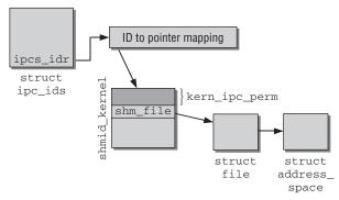
Figure 5-7: Data structures for System V shared memory.
