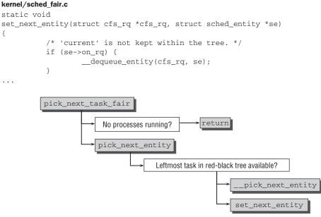
Figure 2-21: Code flow diagram for pick\_next\_task\_fair.
