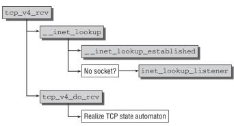
Figure 12-27: Code flow diagram for tcp\_v4\_rcv.
