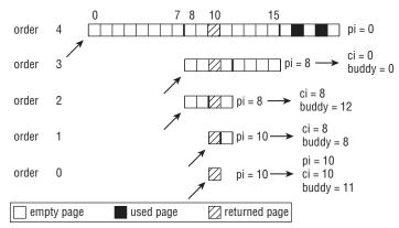
Figure 3-36: Returning a page into the buddy system can cause higher-order allocations to be coalesced. pi stands for page\_index, while ci denotes combined\_index.
