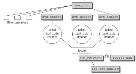
Figure 5-3: The system calls to obtain IPC objects can be unified by a common helper function.
