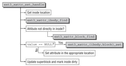
Figure 11-9: Code flow diagram for ext3\_xattr\_set.
