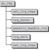
Figure 14-9: Code flow diagram for do\_IRQ. on AMD64 systems.
