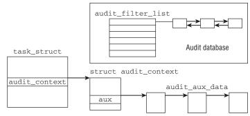
Figure 19-2: Data structures used by the audit mechanism.
