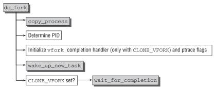
Figure 2-7: Code flow diagram for do\_fork.
