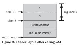
The procedure parameters are found by reference to the frame pointer. The compiler knows that they are located directly at the end of the activation record of the calling function and that two 4-byte
