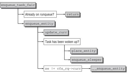
Figure 2-20: Code flow diagram for enqueue\_task\_fair.
