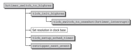
Figure 15-18: Code flow diagram for hrtimer\_switch\_to\_hires.
