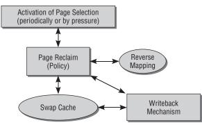
Figure 18-4: Interaction between the swap cache and the other components of the swap subsystem.
