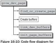
Figure 16-10: Code flow diagram fo grow\_dev\_page.
