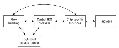
Figure 14-3: Various types of interrupt handlers and how they are connected.
