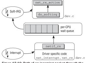
Figure 12-10 shows an overview of the path followed by a packet through the kernel to the network layer functions after it arrives at the network adapter.
