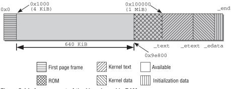
Figure 3-11: Arrangement of the Linux kernel in RAM memory.
