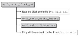
Figure 11-7: Code flow diagram for ext3\_xattr\_block\_get.
