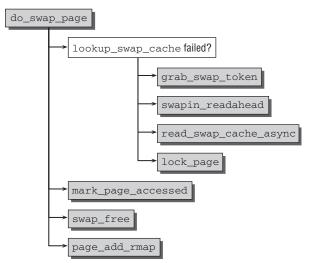
Figure 18-19: Code flow diagram for do\_swap\_page.
