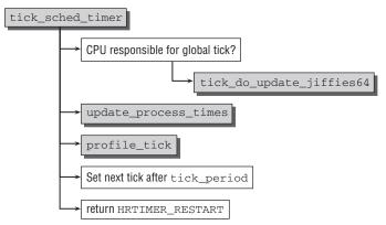
Figure 15-17: Code flow diagram for tick\_sched\_timer.
