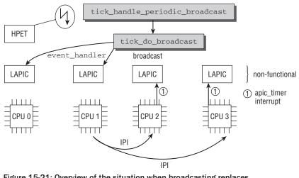
Figure 15-21: Overview of the situation when broadcasting replaces nonfunctional tick devices.
