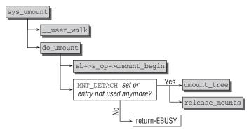
Figure 8-8: Code flow diagram for sys\_umount.
