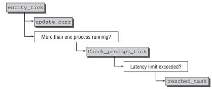
Figure 2-22: Code flow diagram for entity\_tick.
