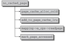
Figure 8-15: Code flow diagram for no\_cached\_page.
