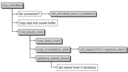
Figure 12-31: Code flow diagram for tcp\_sendmsg.
