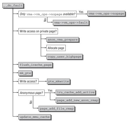
Figure 4-19: Code flow diagram for \_\_do\_fault.
