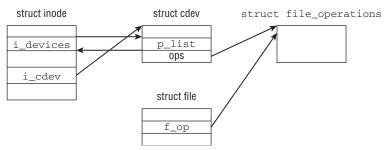
Figure 6-7: Relations between data structures for the representation of character devices.
