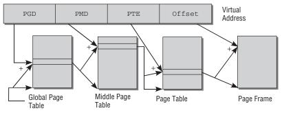
Figure 1-7: Splitting a virtual address.
