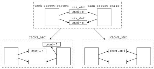
Figure 2-10: When a new thread is created, resources of the parent can either be shared or copied.
