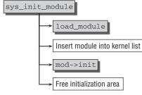
Figure 7-4: Code flow diagram for sys\_init\_module.
