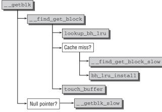
Figure 16-9: Code flow diagram for <u>\_\_getblk</u>.
