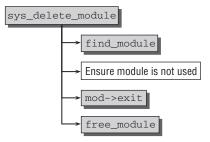
Figure 7-6: Code flow diagram for sys\_delete\_module.
