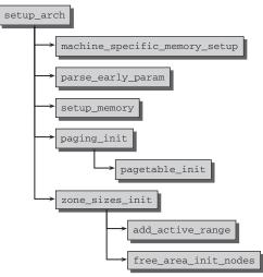
Figure 3-12: Code flow diagram for memory initialization on IA-32 systems.
