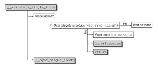
Figure 17-7: Code flow diagram for \_\_writeback\_single\_inode.
