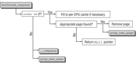
Figure 3-32: Code flow diagram for buffered\_rmqueue.
