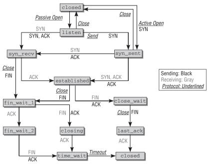
Figure 12-25: TCP state-transition diagram.
