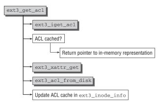
Figure 11-10: Code flow diagram for ext3\_get\_acl.
