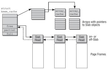
Figure 3-45: Fine structure of a slab cache.
