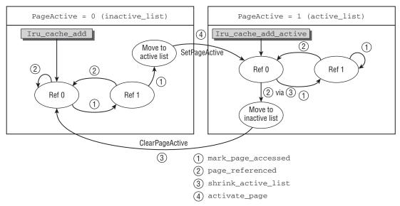
Figure 18-13: Overview of possible state transitions of a page with respect to PG\_active and PG\_referenced, and the corresponding placement of the page on the active and inactive lists.
