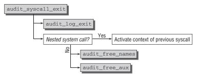
Figure 19-9: Code flow diagram for audit\_syscall\_exit.
