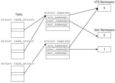
Figure 2-4: Connection between processes and namespaces.
