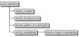
Figure 12-34: Code flow diagram for sys\_sendto.
