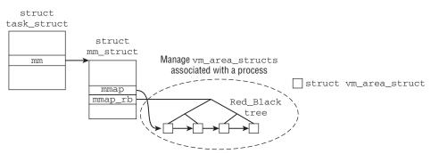
Figure 4-6: Association of vm\_area\_struct instances with the virtual process space of a process.
