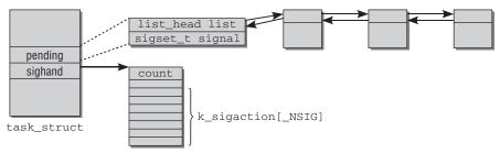
Figure 5-8: Data structures used in signal management.
