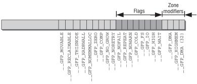
Figure 3-29: Layout of a GFP mask.
