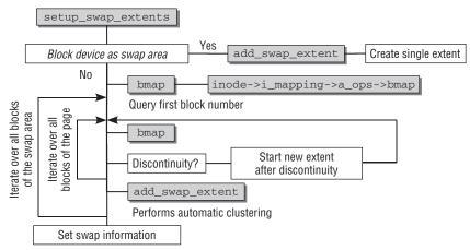
Figure 18-3: Code flow diagram for setup\_swap\_extents.
