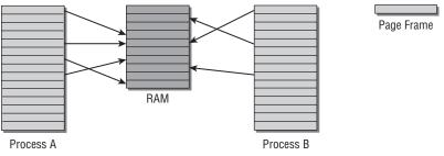
Figure 1-6: Virtual and physical addresses.
