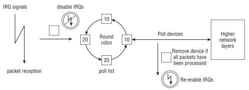
Figure 12-12: Overview of the NAPI mechanism and the round robin poll list.
