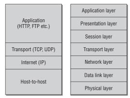
Figure 12-1: TCP/IP and ISO/OSI reference models.
