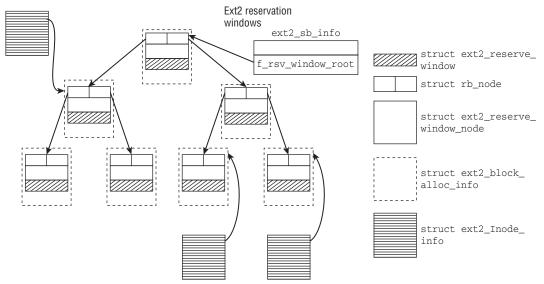
Figure 9-7: Data structures used by the pre-allocation mechanism.
