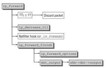
Figure 12-17: Code flow diagram for ip\_forward.
