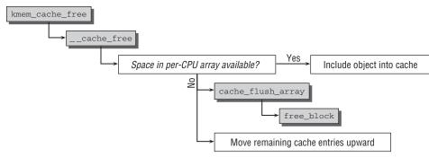
Figure 3-52: Code flow diagram for kmem\_cache\_free.
