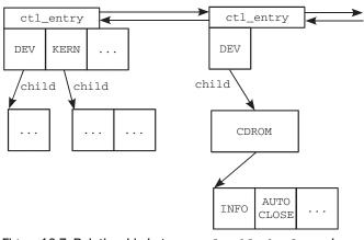
Figure 10-7: Relationship between ctl\_table\_header and ctl\_table.
