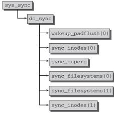
Figure 17-10: Code flow diagram for sys\_sync.
