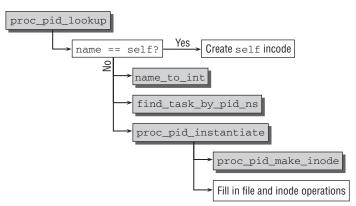
Figure 10-4: Code flow diagram for proc\_pid\_lookup.
