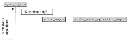
Figure 17-5: Code flow diagram for sync\_supers.
