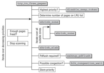
Figure 18-22: Code flow diagram for try\_to\_free\_pages.
