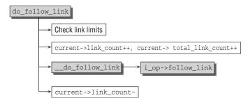
Figure 8-10: Code flow diagram for do\_follow\_link.
