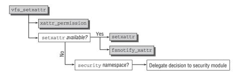
Figure 11-3: Code flow diagram for vfs\_setxattr.
