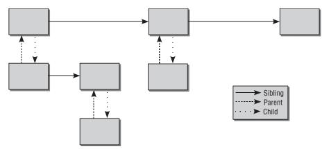
Figure 6-20: Resource management in a tree structure.
