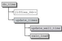
Figure 15-5: Code flow diagram for do\_time.
