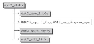
Figure 9-18: Code flow diagram for ext2\_mkdir.
