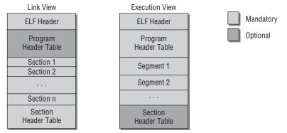
Figure E-1: Basic layout of ELF files.
