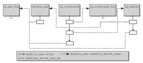
Figure 7-3: Data structures for managing dependencies between modules.
