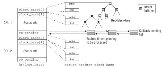
Figure 15-12: Overview of the data structures used to implement high-resolution timers.
