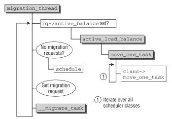
Figure 2-27: Code flow diagram for migration\_thread.
