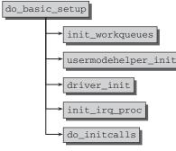
Figure D-4: Code flow diagram for do\_basic\_setup.
