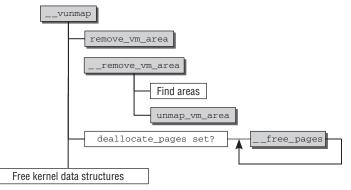
Figure 3-40: Code flow diagram for \_\_vunmap.
