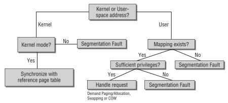
Figure 4-17: Potential options for handling page faults.
