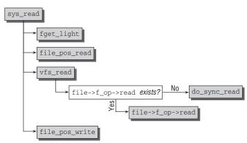
Figure 8-12: Code flow diagram for sys\_read.
