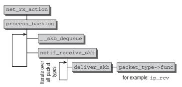
Figure 12-11: Code flow diagram for net\_rx\_action.
