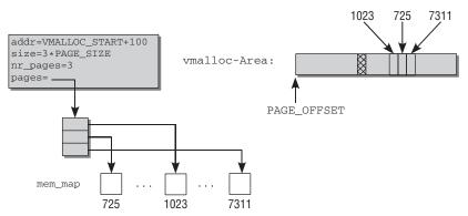
Figure 3-38: Mapping physical pages into the vmalloc area.
