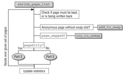
Figure 18-17: Code flow diagram for shrink\_page\_list (Part 1)
