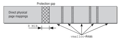
Figure 3-37: vmalloc area in the kernel's virtual address space on IA-32 systems.
