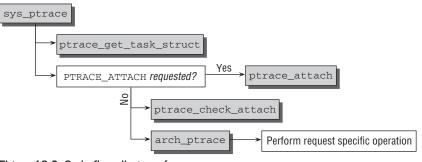
Figure 13-2: Code flow diagram for sys\_ptrace.
