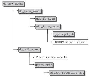
Figure 8-6: Code flow diagram for do\_new\_mount.
