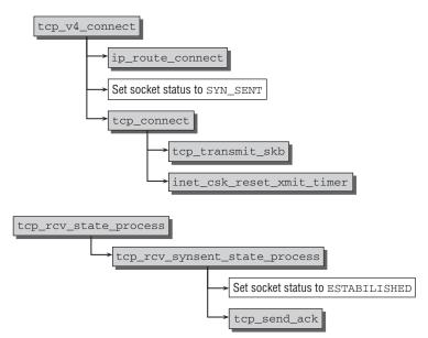
Figure 12-29: Code flow diagram for active connection establishment.
