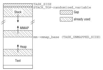
Figure 4-1: Composition of the linear process address space.
