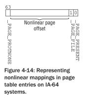
Swap identifiers are 64 bits long. Bit 0 must be zero because the page is not present, and bit 1 represents \_PAGE\_FILE to indicate that the entry belongs to a nonlinear mapping in contrast to a swap specifier. The last bit, that is, 63, is reserved for the \_PAGE\_PROTNONE bit.<sup>12</sup> Consequently, this leaves 61 bits raw capacity to represent the nonlinear page offset.
