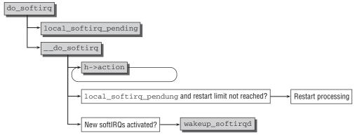
Figure 14-11: Code flow diagram for do\_softirg.
