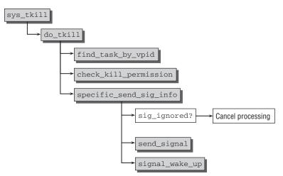
Figure 5-9: Code flow diagram for sys\_tkill.
