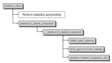
Figure 6-16: Code flow diagram for submit\_bio.
