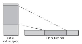
Figure 4-4: Mapping a file into virtual memory.
