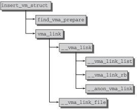
Figure 4-11: Code flow diagram for insert\_vm\_struct.
