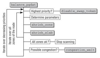
Figure 18-21: Code flow diagram for balance\_pgdat.
