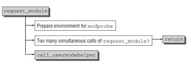
Figure 7-7: Code flow diagram for request\_module.
