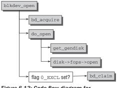
Figure 6-13: Code flow diagram for blkdev\_open.
