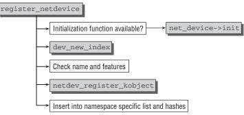
Figure 12-9: Code flow diagram for register\_netdevice.
