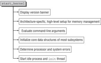
Figure D-1: Code flow diagram for start\_kernel.
