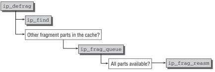
Figure 12-16: Code flow diagram for ip\_defrag.
