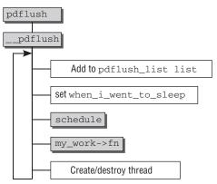
Figure 17-3: Code flow diagram for pdflush.
