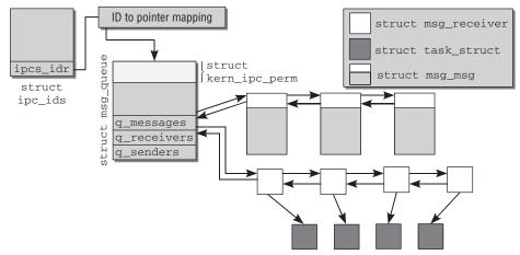
Figure 5-6: Data structures for System V message queues.
