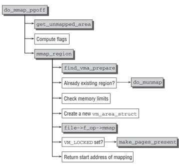
Figure 4-12: Code flow diagram for do\_mmap\_pgoff.
