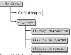
Figure 17-12: Code flow diagram for \_\_\_do\_sync.
