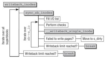
Figure 17-6: Code flow diagram for writeback\_inodes.
