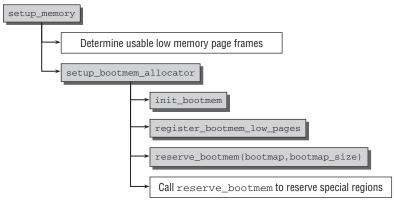
Figure 3-20: Initialization of the bootmem allocator on IA-32 machines.
