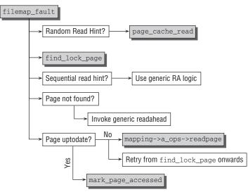
Figure 8-16: Code flow diagram for filemap\_fault.
