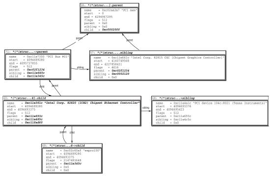
Figure 6-21: Allocated resources of a PCI network card.
