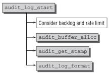
Figure 19-5: Code flow diagram for audit\_log\_start.
