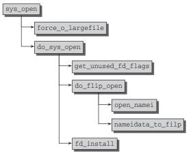
Figure 8-11: Code flow diagram for sys\_open.
