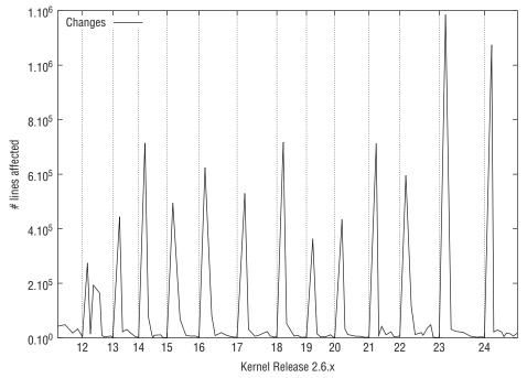
Figure F-1: Rate of change in the vanilla kernel. An open merge window leads to a rapid burst of changes, followed by a stabilization period with a considerably smaller change rate.
