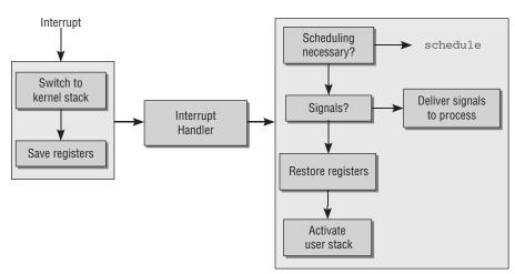
Figure 14-2: Handling an interrupt.
