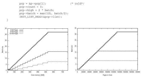
Figure 3-17: Batch sizes dependent on the amount of memory present (left-hand side) on the zone for various page sizes. The graph on the right-hand side shows the dependency against the number of pages present in a zone.
