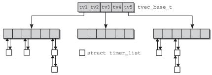
Figure 15-6: Data structures for managing timers.
