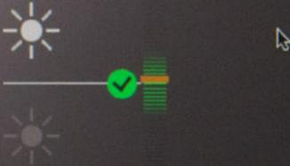
Adjust your display's brightness or backlight control until the measured luminance is as close as possible to the target. If your display cannot be adjusted low enough, i1Profiler will automatically match the target luminance when building the profile. When you are finished making adjustments (or if your display does not have a brightness control), press "Next" to continue.
